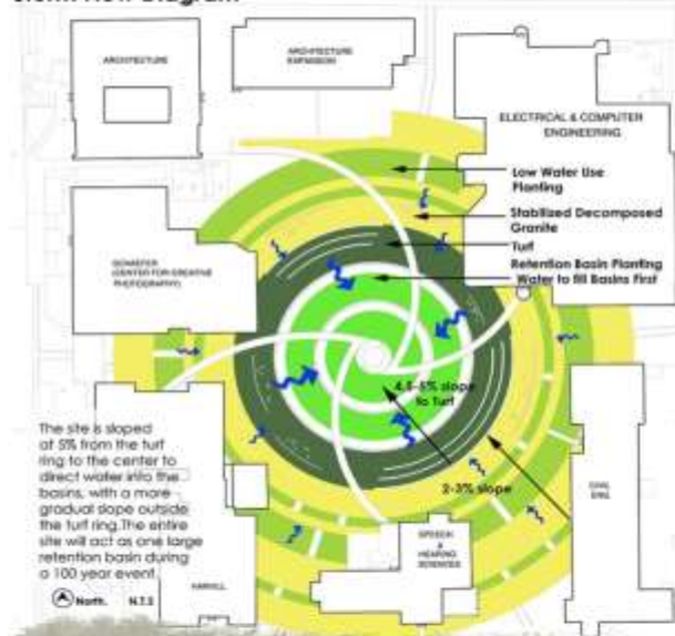
Storm Flow Diagram
